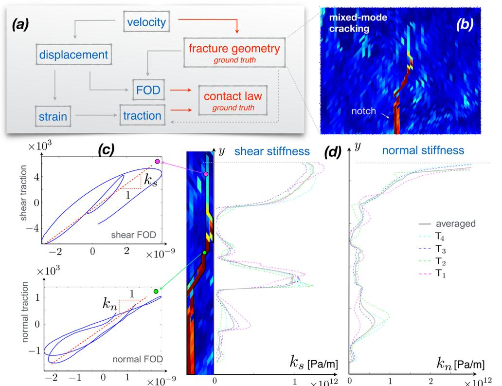
Fig.4 : Full-field characterization of the fracture geometry and heterogeneous interfacial condition: (a) roadmap, (b) reconstructed geometry, (c) contact law, (d) heterogeneous distribution of the specific stiffness in shear and normal directions
