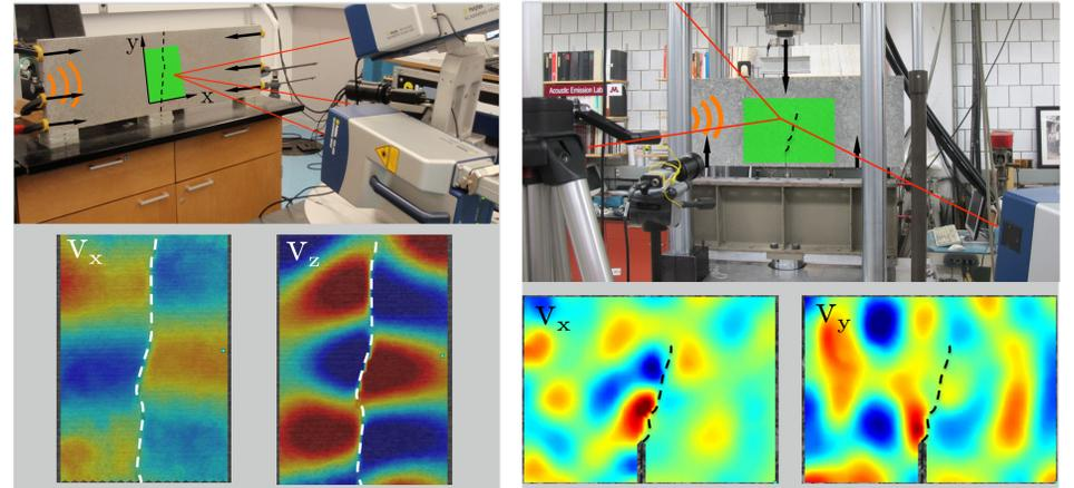
Fig.3 : SLDV setup for full-field ultrasonic sensing of stationary and evolving fractures in rock
