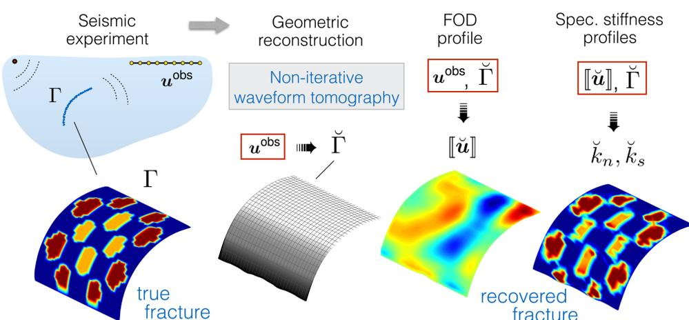
Fig. 2 Three-step approach to holistic seismic sensing of heterogeneous fractures
