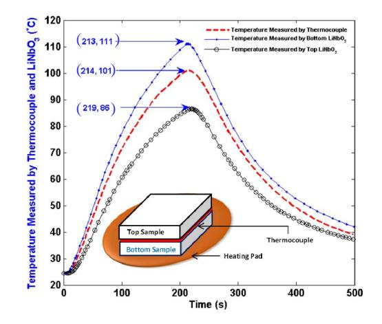
Temperature measured by the thermocouple and 1 mm thick sandwich structured LiNbO<sub>3</sub>
