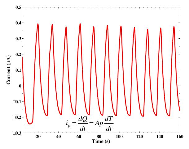
Current generated from LiNbO <sub>3</sub> with continuous heating and cooling
