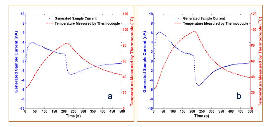
Generated current by LiNbO<sub>3</sub> and temperature of thermocouple mounted on top of (a) 2 mm thick LiNbO<sub>3</sub> and (b) 1 mm thick LiNbO<sub>3</sub>
