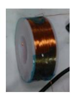
Length .017 m Inner radius .0127 m Outer radius .02413 m Number turns 6740 Magnetic wire resistance 1100 ohm
