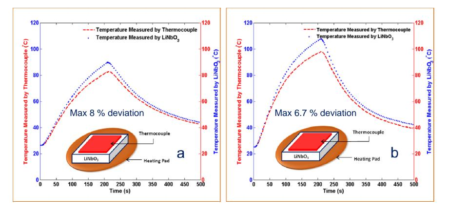
Temperature measured by thermocouple and (a) 2 mm thick and (b) 1 mm thick LiNbO $_3$
