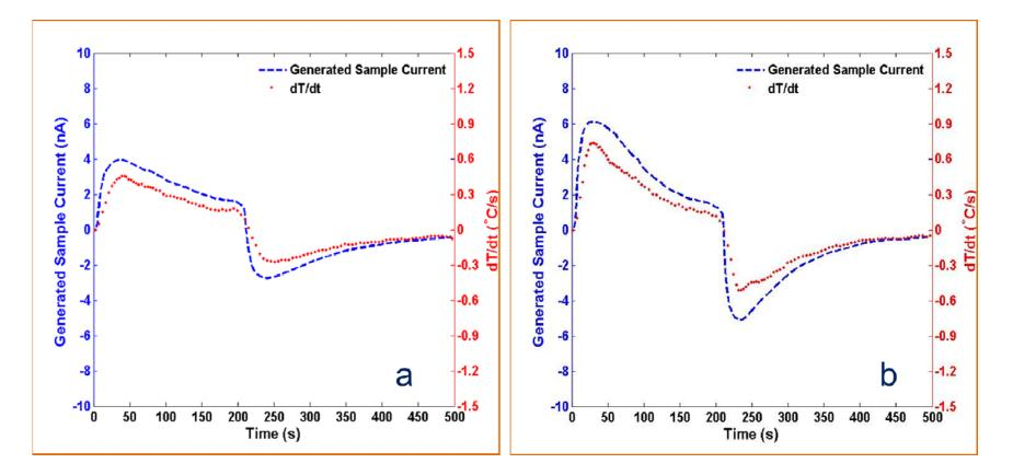
Generated current by LiNbO<sub>3</sub> and rate of temperature change of thermocouple mounted on top of (a) 2 mm and (b) 1 mm thick LiNbO<sub>3</sub>
