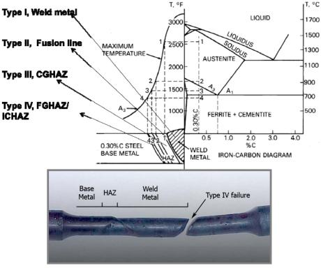
Weld Joint Strength Reduction Factors (WSRF =  $\sigma_{weld} / \sigma_{base metal}$ ) for CSFE steels can be as low as 0.5 at ~600°C.
