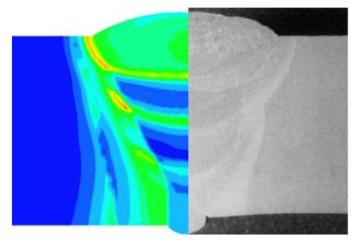
Yield strength gradient simulation in a multi-pass steel weld
