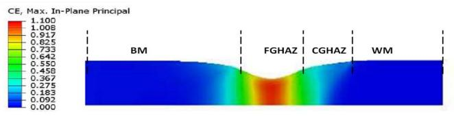
Figure 1. Maximum in-plane creep strain in a cross-weld specimen after 13000 hours creep. (CE is in-plane principal creep strain)
