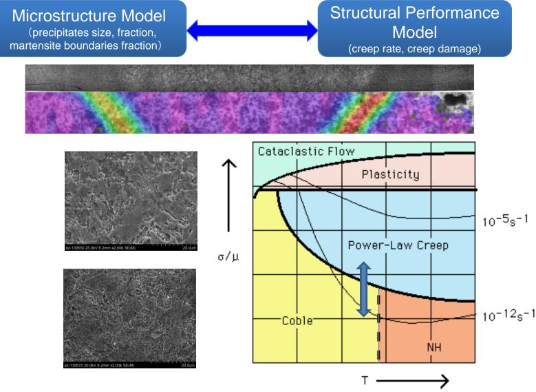
0.1mm deformation mechanism map
