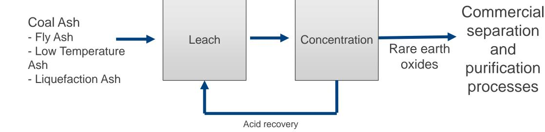
Integrated bench scale system design for potential phase 2
