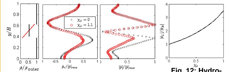
Figure 11: Hydrodynamic mode shapes with and without asymmetry.
