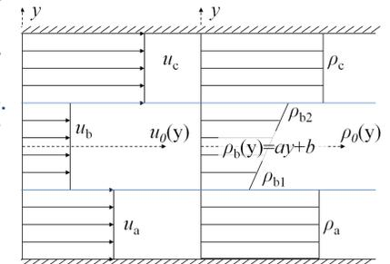
Figure 9: Generalized model profiles for base velocity (left) and base density (right)
