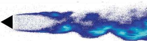
Figure 4: Reacting bluff body flowfield exhibiting base density asymmetry
