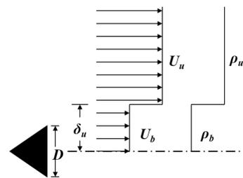
Figure 1: Velocity and Density profile for reacting bluff body wake (1)
