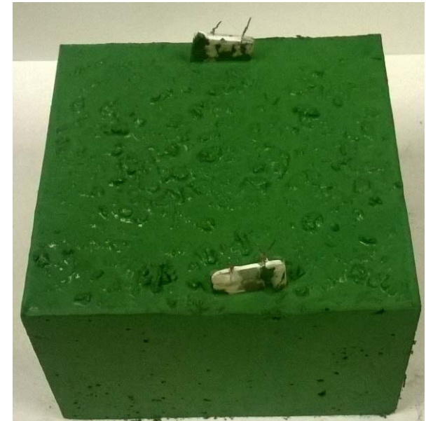
Chromia brick showing exposed sensor preform.
