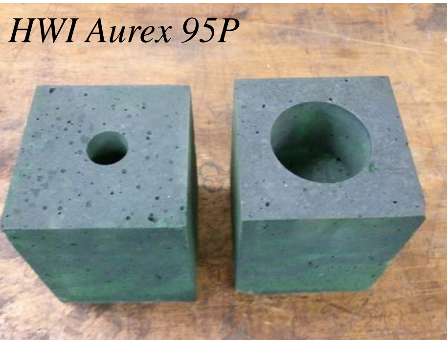
Fired high-chromia brick with sensor (thermistor).
