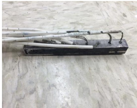
9 type-K thermocouples were attached to the steel bar at an equal spacing.
