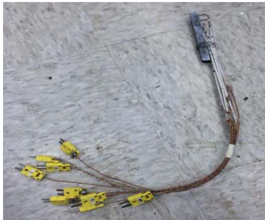
9 type-K thermocouples were attached to the steel bar at an equal spacing.
