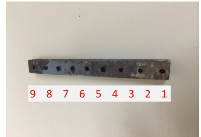
The steel bar was placed to an open end tube furnace at 1000°C (center) for 10 hrs.
