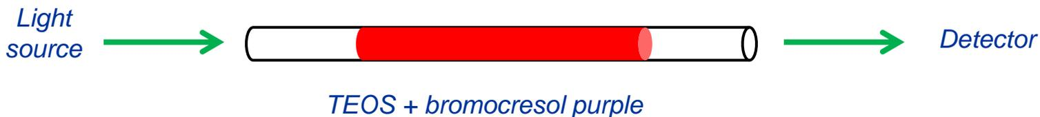
**pH Indicators Can Also Be Embedded within a Sol-Gel Matrix Such as Silica and Integrated with a Fiber Optic Based Sensing Platform**
