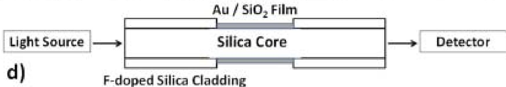
**Sensor Elements Have Been Fabricated Based upon the Au / SiO<sub>2</sub> System to Explore High Temp. Plasmonic Sensing Exploiting Au LSPR Absorption Modifications.**
