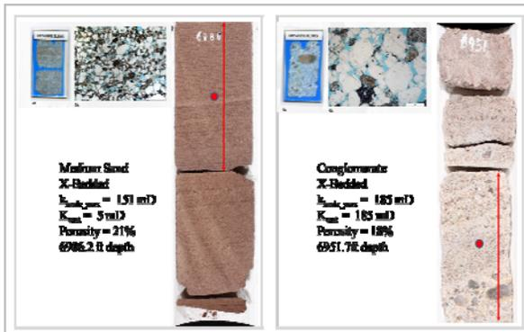
**Figure 1** Core samples, thin sections, and photomicrographs from the Lower Mt. Simon Sandstone reservoir.
