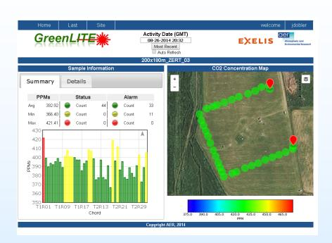
ZERT test results showed that the 2D reconstruction algorithms could see persistent features from both the controlled release and from a large manure pile in the Northeast corner, but wind and natural variation in background make independent validation of reconstructions challenging.
