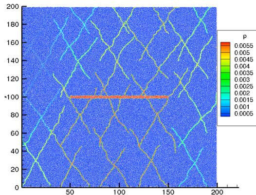
Fluid pressure distribution after flow reached steady-state
