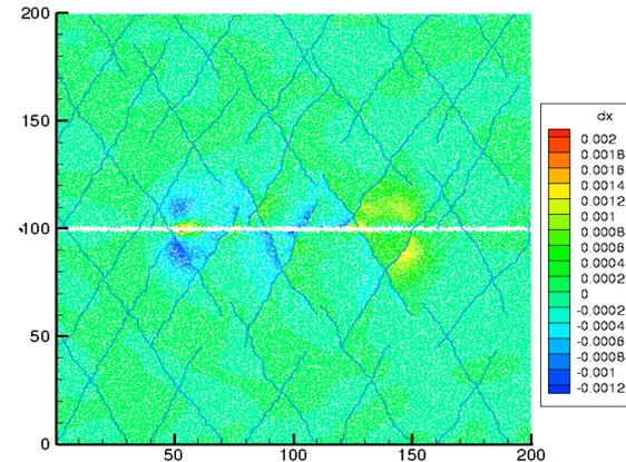
Horizontal displacement field and fracture network colored by fracture permeability
