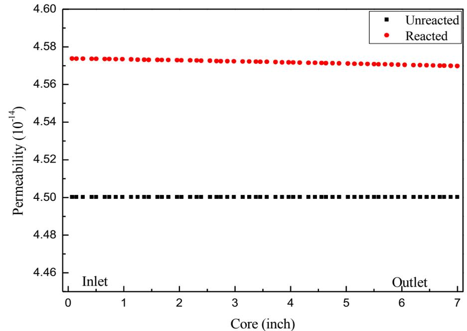
Slightly larger changes at the inlet. Maximum amount is predicted to be 0.5 % and 1.4 % for porosity and permeability, respectively. This is consistent with experimental data.
