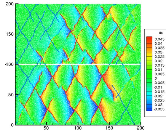
Horizontal displacement field and fracture network colored by fracture permeability
