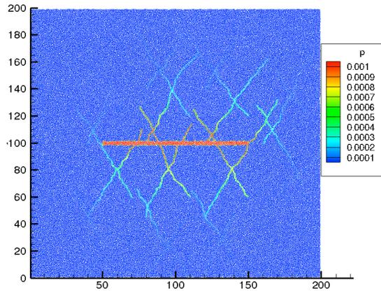
Fluid pressure distribution shortly after the injection was started
