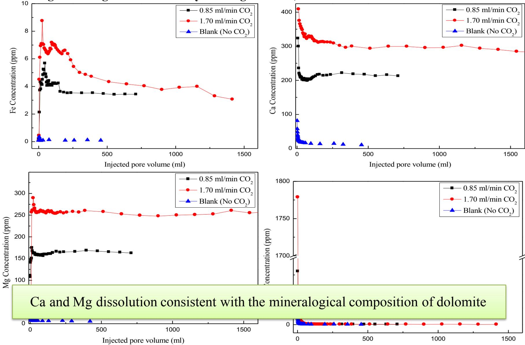
Ca and Mg dissolution consistent with the mineralogical composition of dolomite
