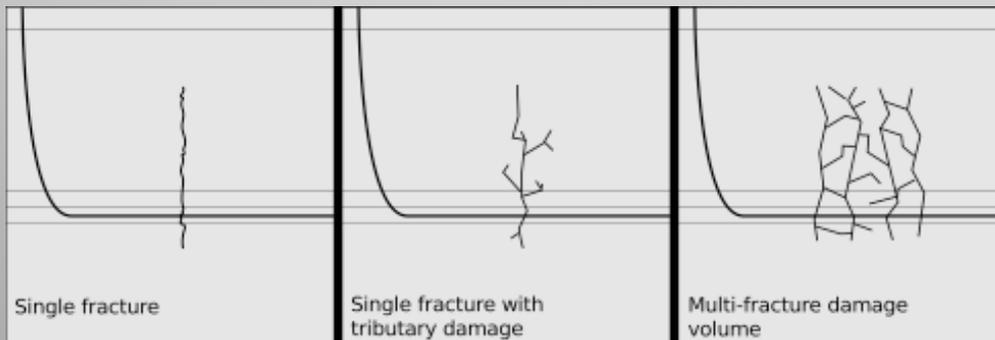
Spectrum of fracture behavior, from single mode-I fracture to a complex multi-fracture environment
