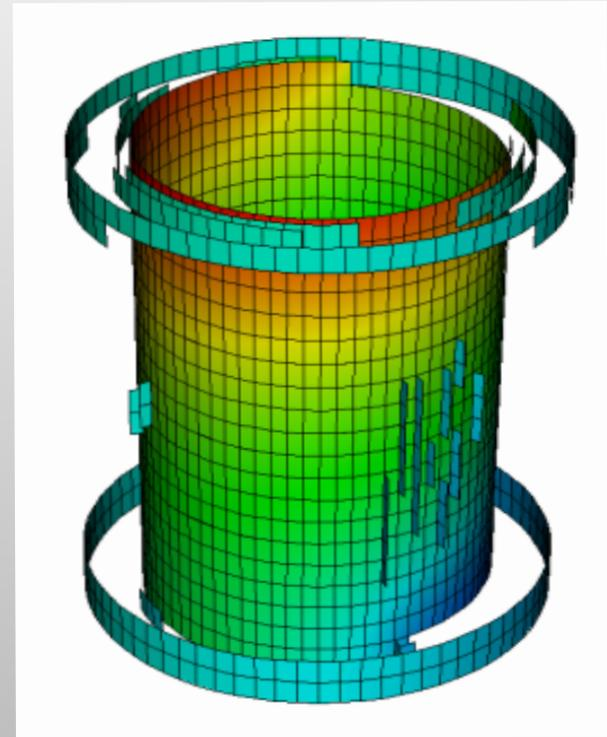
Adding confining pressure slows fracture propagation
