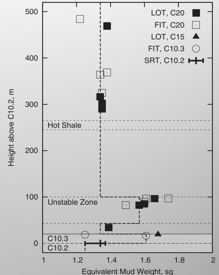
In Salah leak off test and formation integrity test data.
