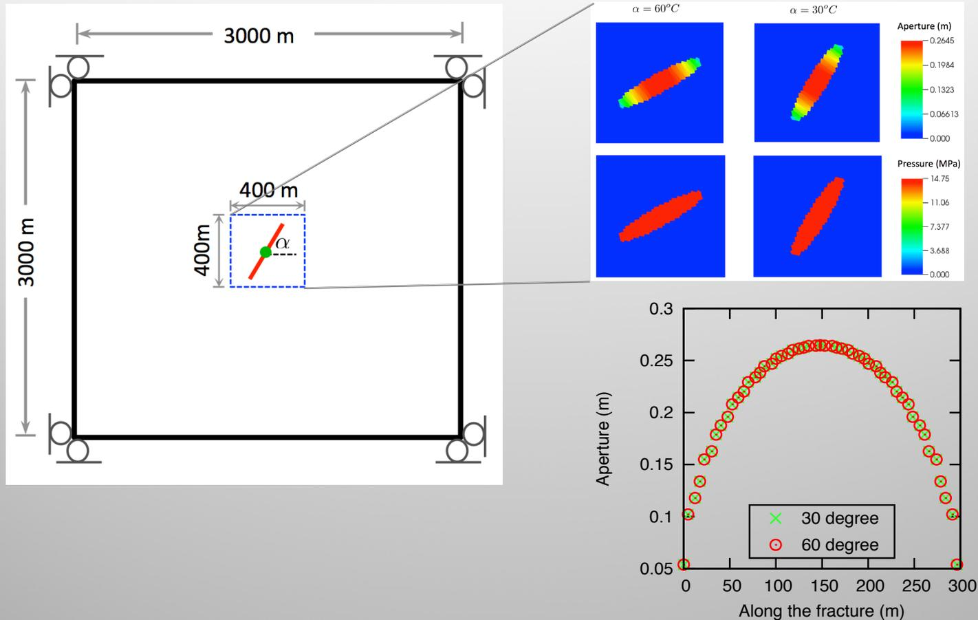
Simple test problem with a pressurized crack on a fixed background mesh. Computed response is independent of crack orientation, as expected.
