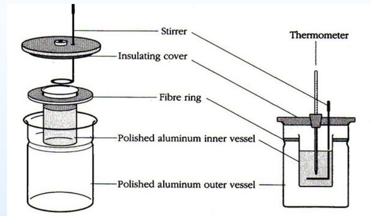
Figure 2.1.1. The components of a calorimeter (MiniScience.com).
