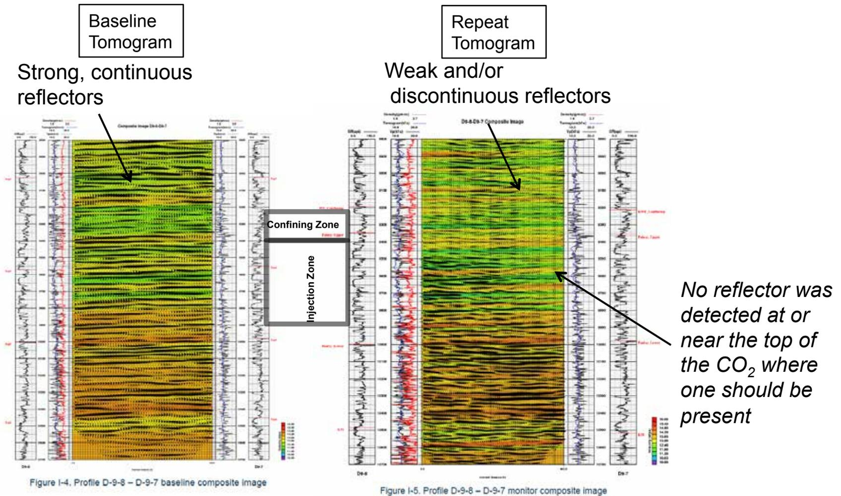
Reflection data from the repeat survey are of poor quality and limited use. Likely cause is interference by tube waves moving up and down the well
