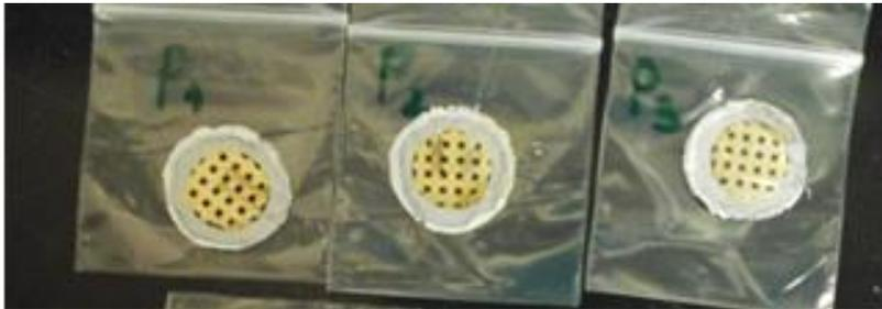
Full cells with Au grid after the measurements.
