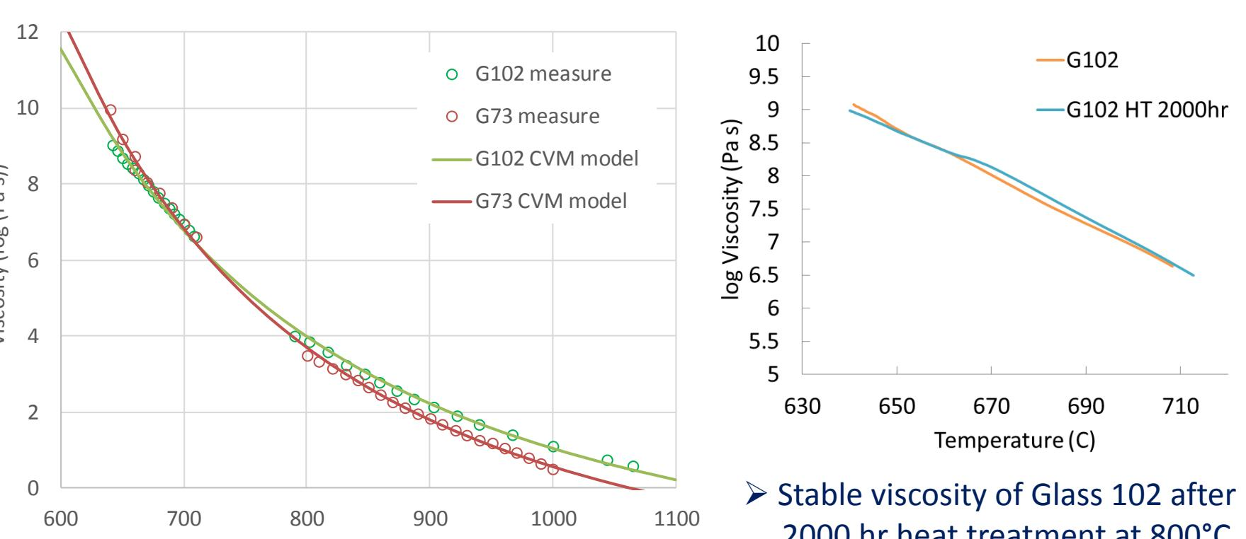
Stable viscosity of Glass 102 after 2000 hr heat treatment at 800°C
