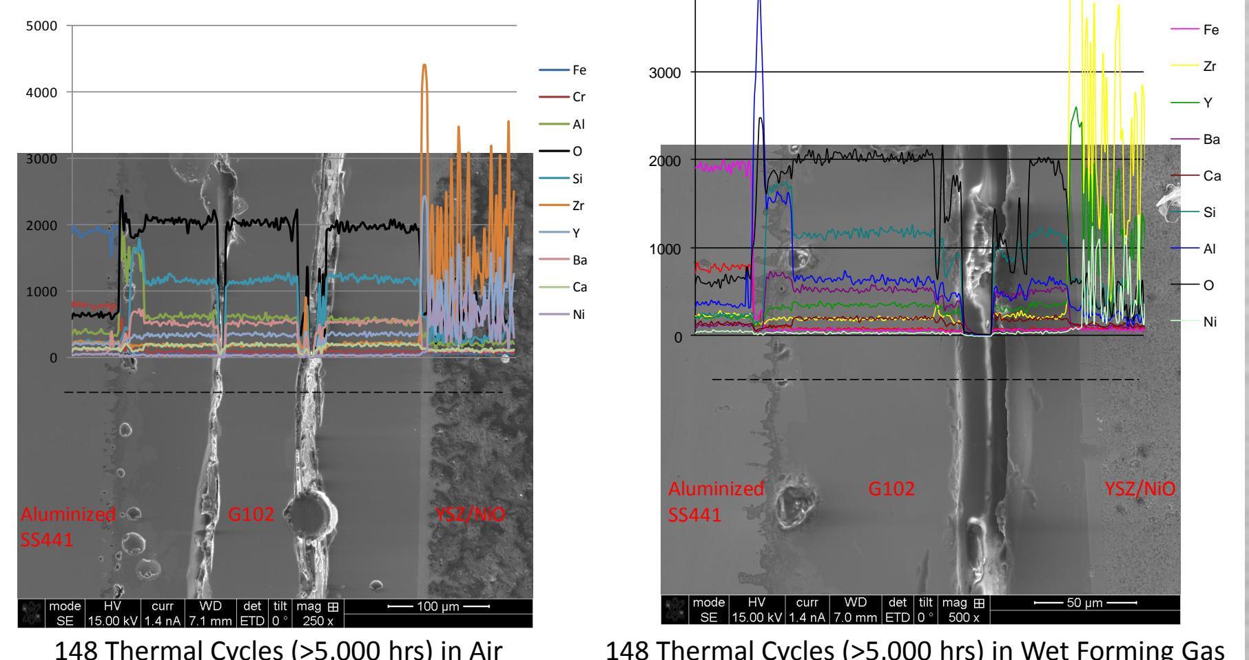
148 Thermal Cycles (>5,000 hrs) in Air
