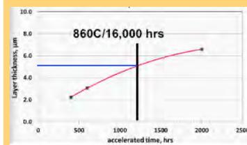
Prior results [1] from LGFCs on thickness of densified cathode layer vs. duration of accelerated testing. The vertical black line indicates that 1.2 kh under the accelerated conditions produced the same thickness of densified cathode (5 µm) as was observed after 16 kh of testing under simulated system conditions (horizontal blue line).
