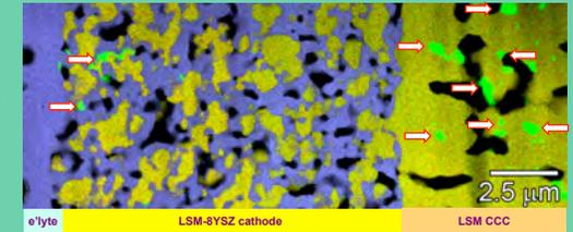
•  $MnO_x$  near cathode-electrolyte interface & in CCC
