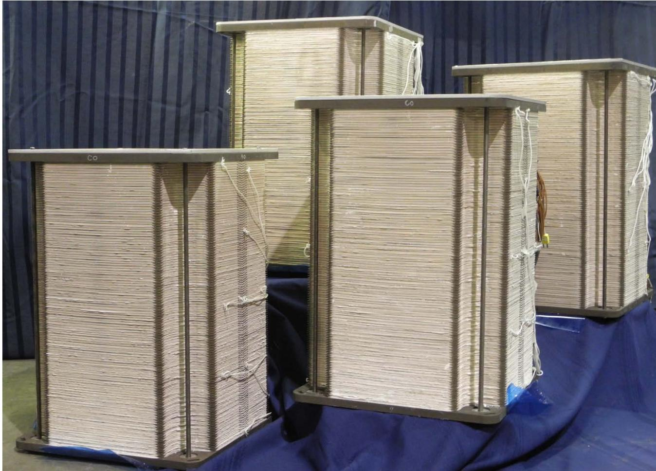
**Recently, four 120-cell stacks were built and conditioned to be utilized in a 50 kW Proof-of-Concept System Tests**
