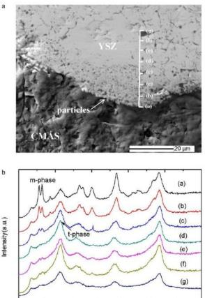
Fig. 4. (a) Micrograph of the interaction zone of CMAS deposit and YSZ coating after 4 h heat-treatment at 1250 °C, and (b) Raman spectra obtained from the positions marked in (a).
