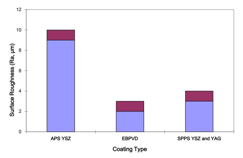
A smoother surface provides aerodynamic, heat transfer and erosion resistance benefits.
