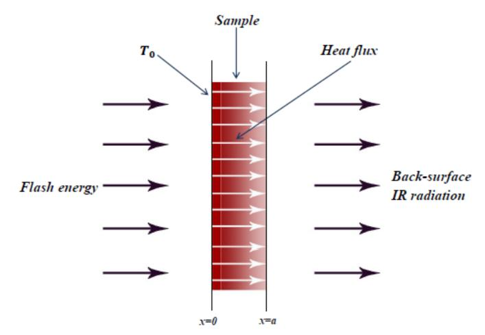
Figure: Diagram of the flash method for measuring thermal diffusivity.
