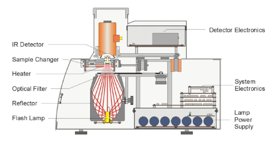
Figure 2: Schematic of the NETZSCH LFA 447
