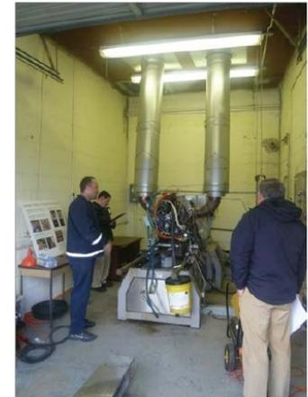
Figure 13 - Turbo-Shaft Test Water Break Dynamometer
