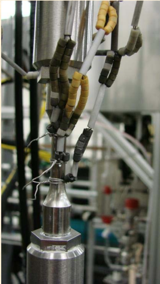
Specimen with three TCs (before exposure)
