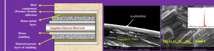
Multiple layers of coatings to interface the embedded sensor and the host and to provide the chemical, thermal, mechanical and optical protections of the embedded sensors.
