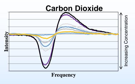
Estimated Detection Limit <sup>12</sup>CO<sub>2</sub> and <sup>13</sup>CO<sub>2</sub> < 1 ppb
