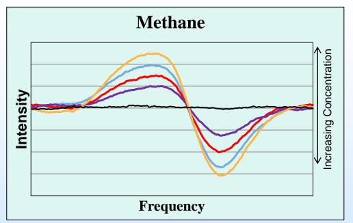
Estimated Detection Limit <sup>12</sup>CH<sub>4</sub> and <sup>13</sup>CH<sub>4</sub> < 1 ppb
