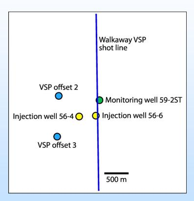
100 shot points along the blue line were used to acquire VSP data recorded at 15 levels of geophone in the monitoring well.
