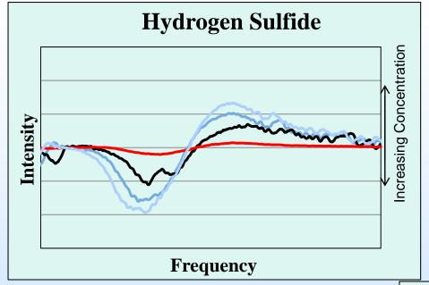
Estimated Detection Limit  $H_2^{32}S < 1 \text{ ppb}$   $H_2^{34}S < TBD$
