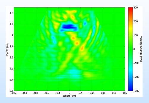
Joint waveform inversion result of time-lapse walkaway VSP data from SACROC reveals a <u>low</u> <u>velocity zone</u> near the CO<sub>2</sub> injection locations.
