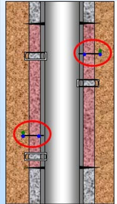
Feet to push O-ring against casing wall
