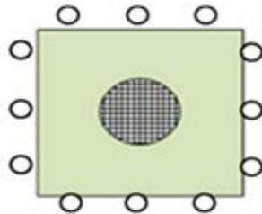
**Step 2- Simulating of drilling step by removing wellbore elements and applying mud weight**
