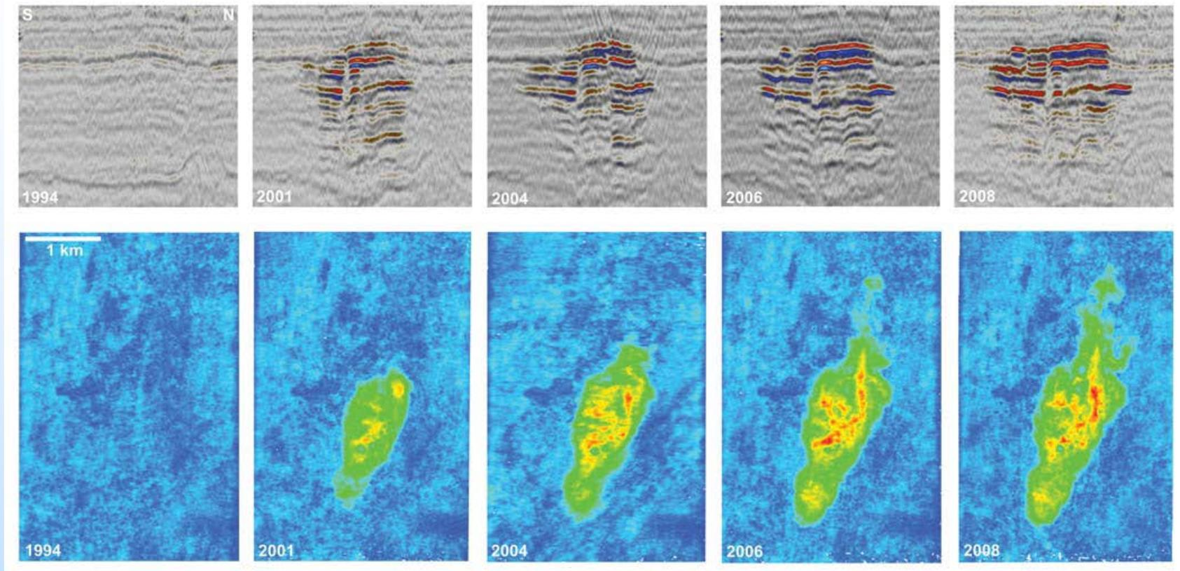
Upper row: N-S seismic section through the plume.
