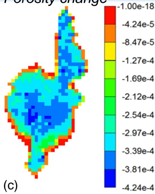
(a) The concentration at the section crossing  $l=33$  (b) distribution at the top sub-layer of Layer 9 in 3D in 2006 (c) distribution at the top sub-layer of Layer 9 in 2006; negative value represents the increase of the porosity due to mineral dissolution.
