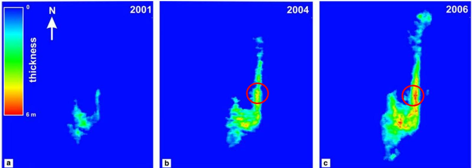
CO<sub>2</sub> plume thicknesses derived from reflection amplitudes (Chadwick and Noy, 2010). A thick area of CO<sub>2</sub> plume (red circle) is clearly shown in 2004 and 2006 map. Propose to add a second feeder to that area after year 2001.
