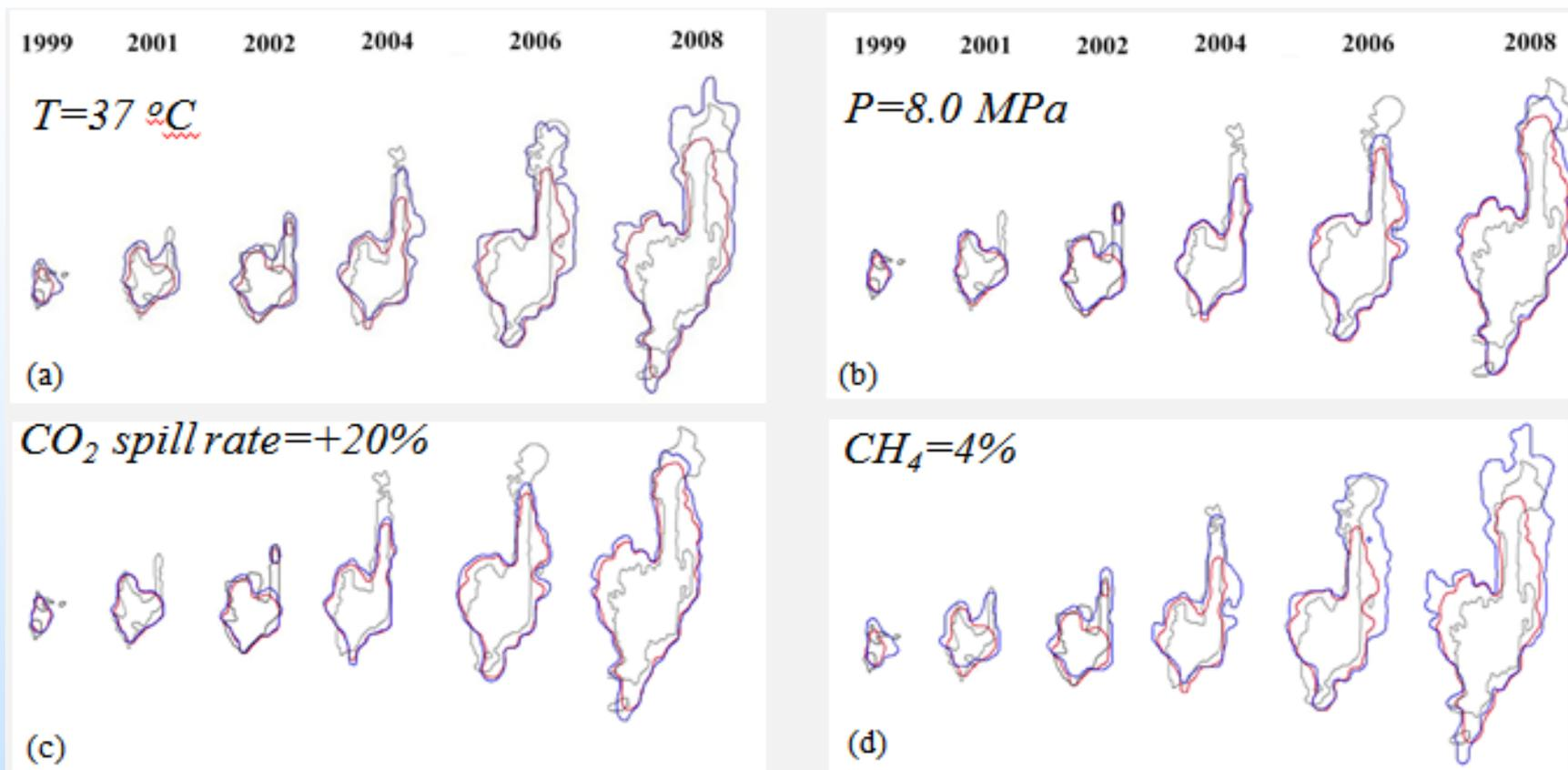
(a)-(d): The black outlines represent CWC observed from 4D seismic (Boait et al., 2012); Red lines represent the Base Case; Blue lines in (a)-(d) represent simulated results of test cases
