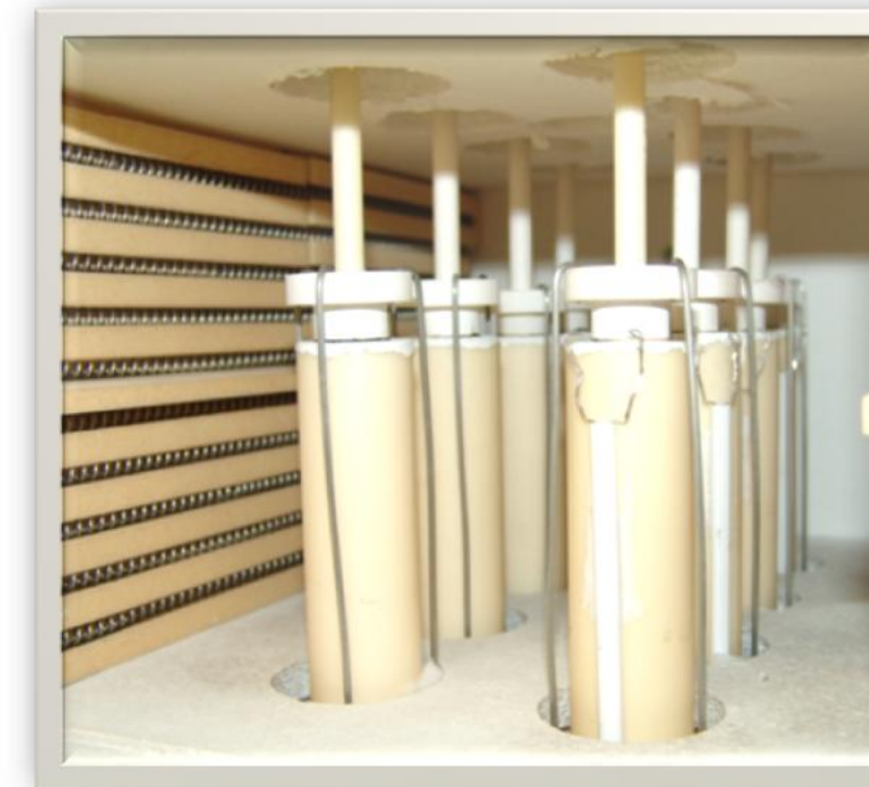
8 button cells installed per box furnace, with individual gas flow controls; 6 furnaces
