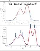
Deconvolution spectrum shows four visible peaks and a shoulder, suggesting the presence of 5 arcs. The equivalent circuit needs 5 arcgenerating elements. The shapes of the peaks guide the choice of arc-generating elements.
