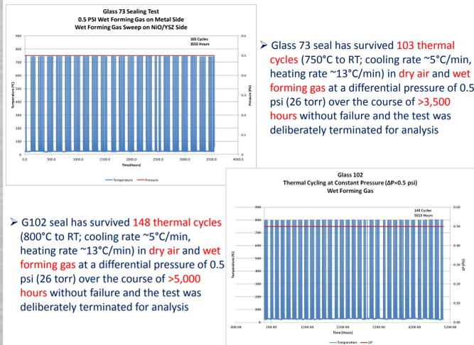
Glass 73 seal has survived **103 thermal cycles** (750°C to RT; cooling rate ~5°C/min, heating rate ~13°C/min) in **dry air** and **wet forming gas** at a differential pressure of 0.5 psi (26 torr) over the course of **>3,500 hours** without failure and the test was deliberately terminated for analysis
