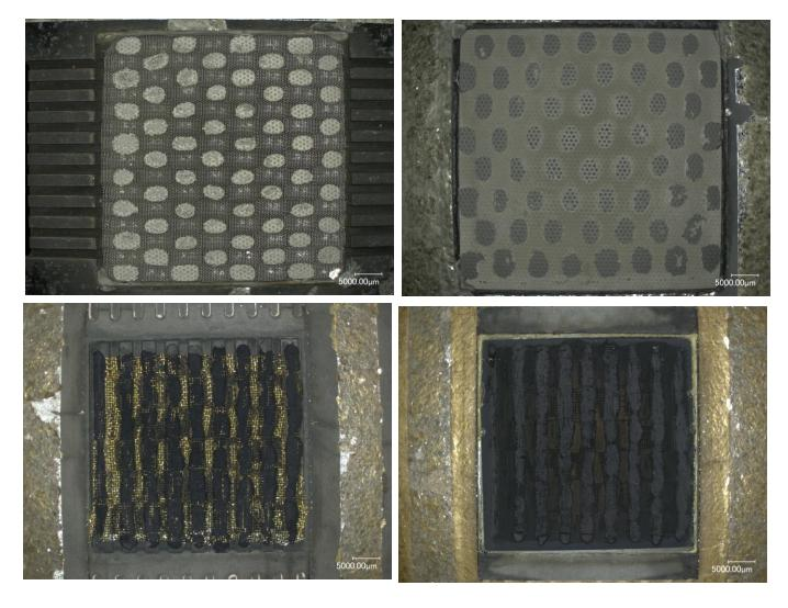
No discoloration on both cathode and anode, consistent with hermetic check with cross-bubbling and iso-propanol penetration. No substantial glass spreading observed.
