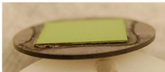
G102 cracked by thermal quenching
