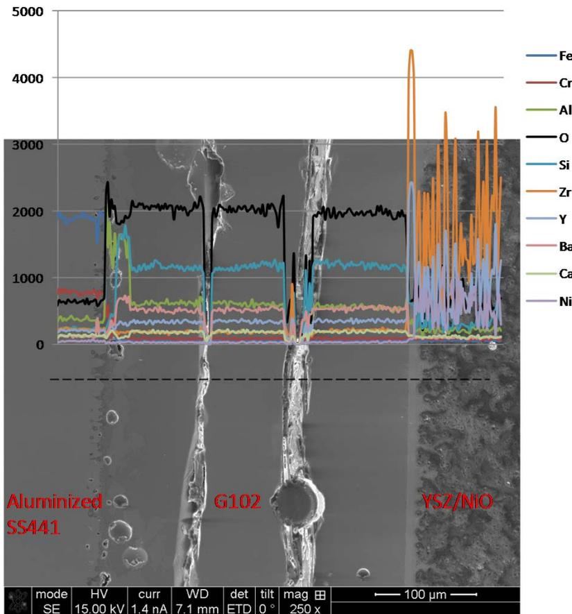
148 Thermal Cycles (>5,000 hrs) in Air
