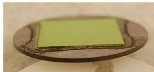
G102 crack healed after re-heating to >744°C for 2 hrs
