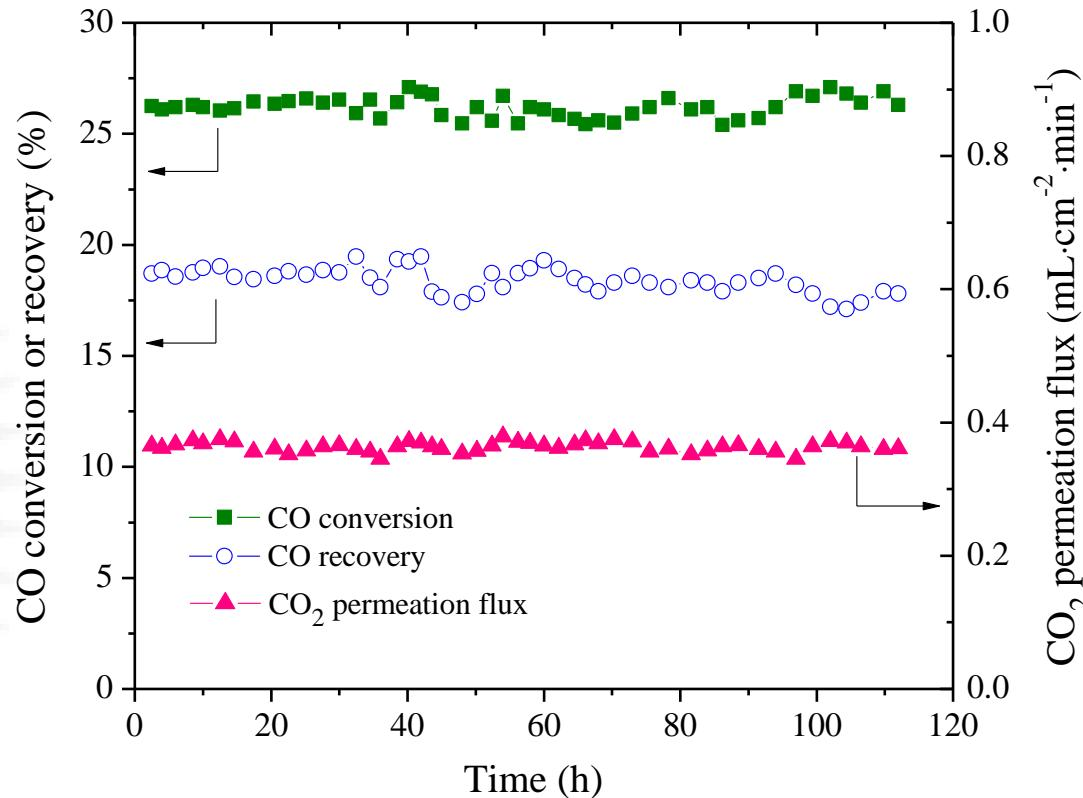
**Long-term stability of the WGS membrane reactor at 900 °C. Syngas flow rate 20 ml/min, H<sub>2</sub>O/CO=3.0.**
