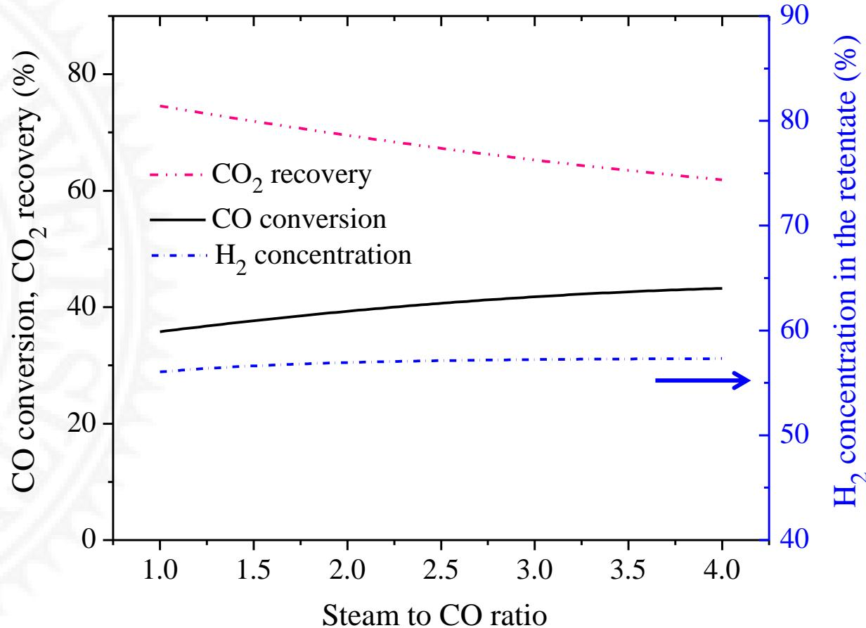
900 °C; 20 atm; Syngas flow rate 25 mL/min.
