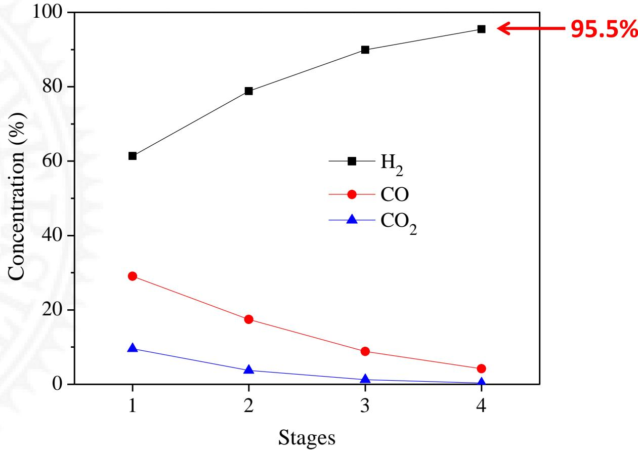
900 °C; 20 atm; syngas flow rate 20 mL/min; Steam to CO ratio of 3.
