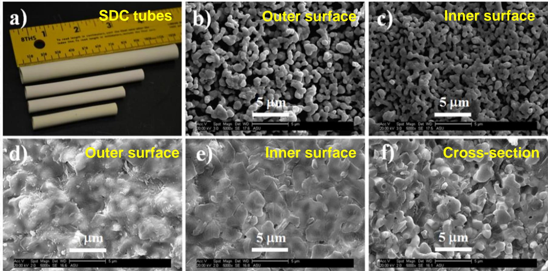
a-c: porous supports; d-f: dual phase membrane
