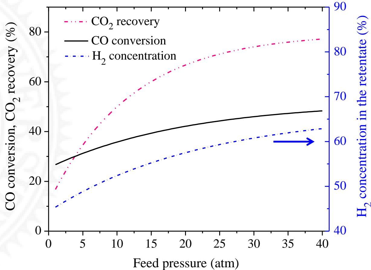
900 °C; Steam to CO ratio of 3; Syngas flow rate 25 mL/min.
