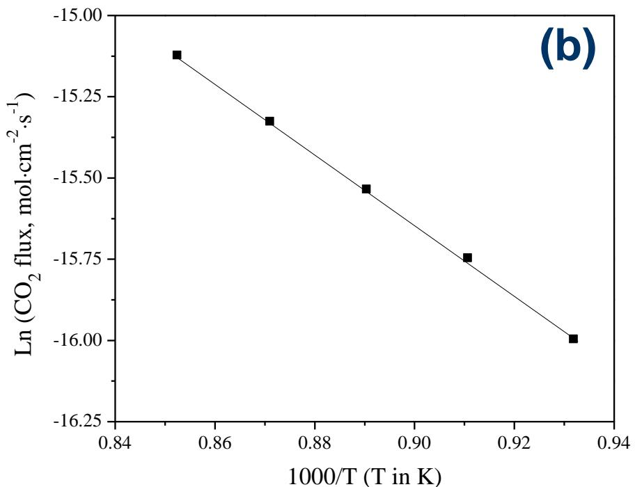
$\text{CO}_2$  flux as a function of temperature during the WGS reaction (a) and the Arrhenius plot (b). Syngas flow rate 20 ml/min,  $\text{H}_2\text{O}/\text{CO}=3.0$ .
