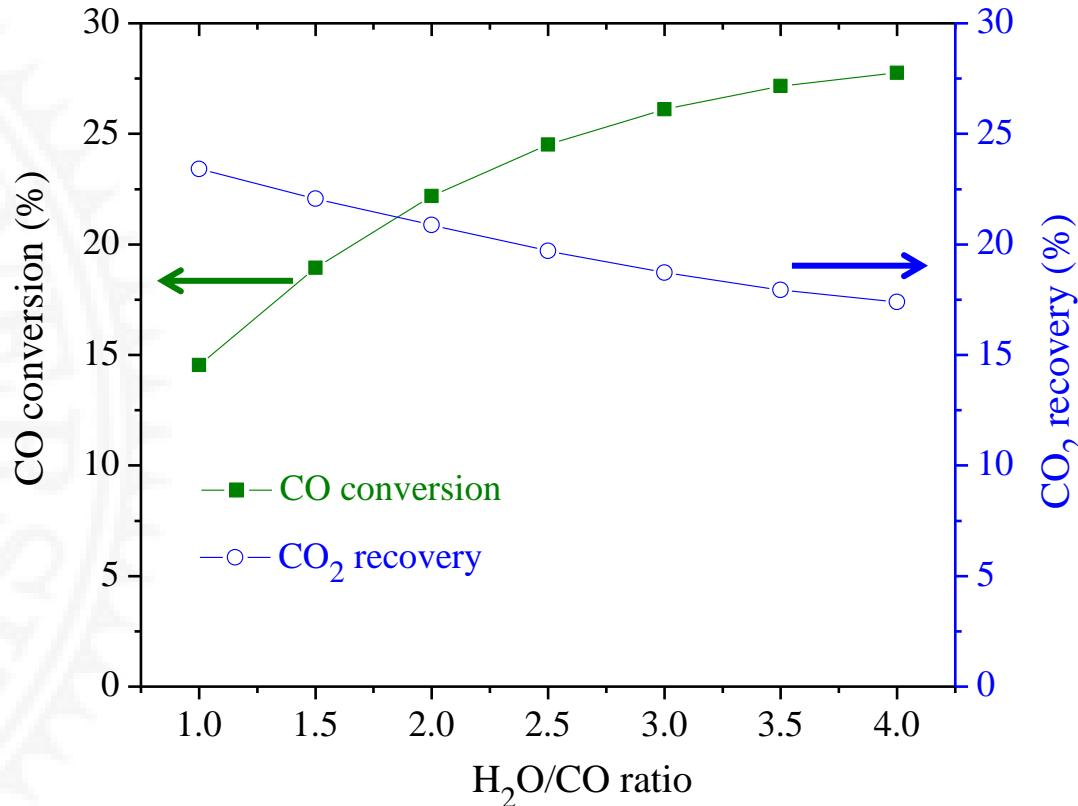
Syngas WGS performance as a function of steam to CO ratio at 900 °C.
