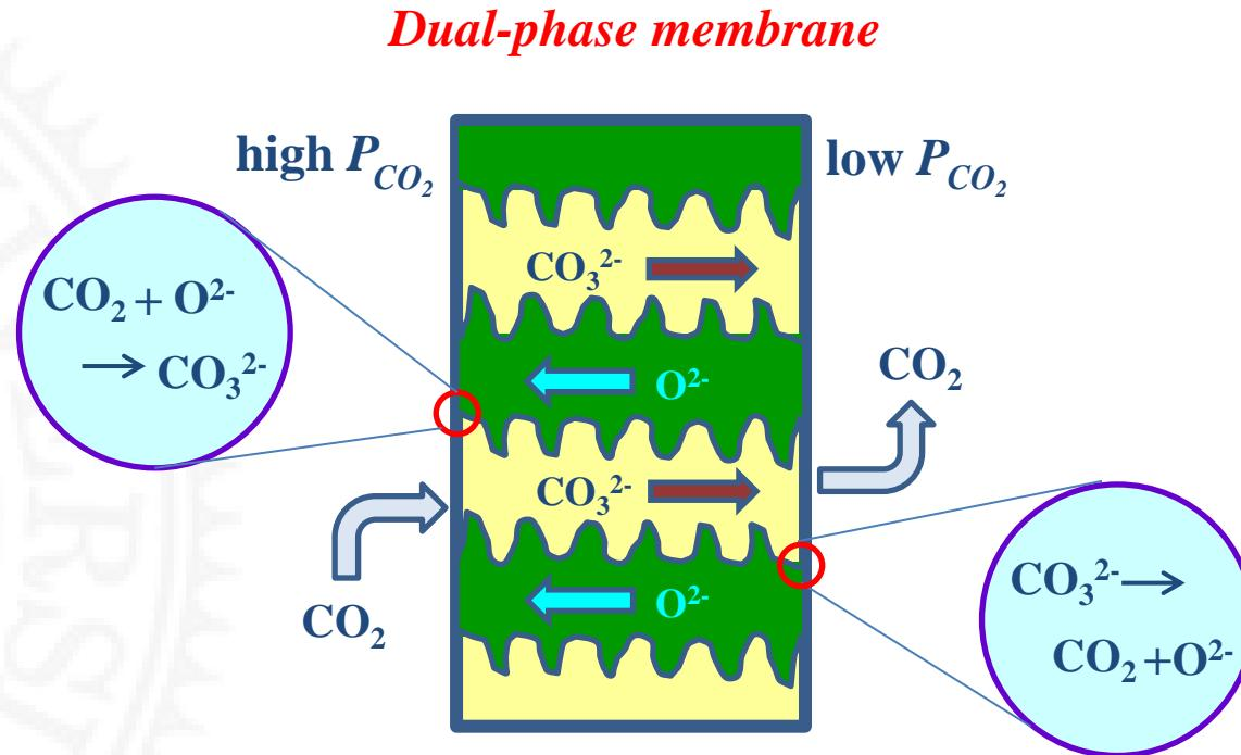
█ Ceramic phase: oxygen ion conductor,  $\text{Sm}_{0.2}\text{Ce}_{0.8}\text{O}_{1.9-\delta}$  (SDC)
