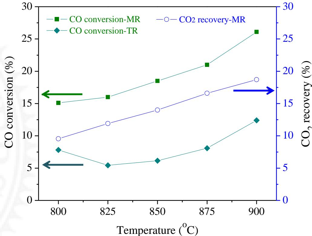
Syngas WGS performance as a function of temperature. Syngas flow rate 20 ml/min; Residence time 1.26 s; H<sub>2</sub>O/CO=3.0.
