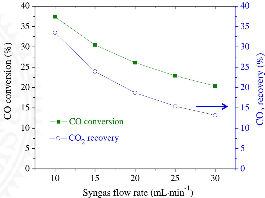
Syngas WGS performance as a function of syngas flow rate at 900 °C.
