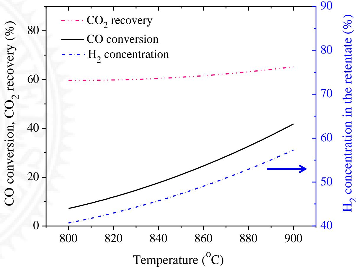
20 atm; Steam to CO ratio of 3; Syngas flow rate 25 mL/min;
