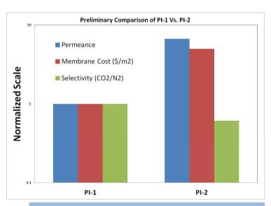
Preliminary Lab testing shows similar trend as PI-1 at low temperature
