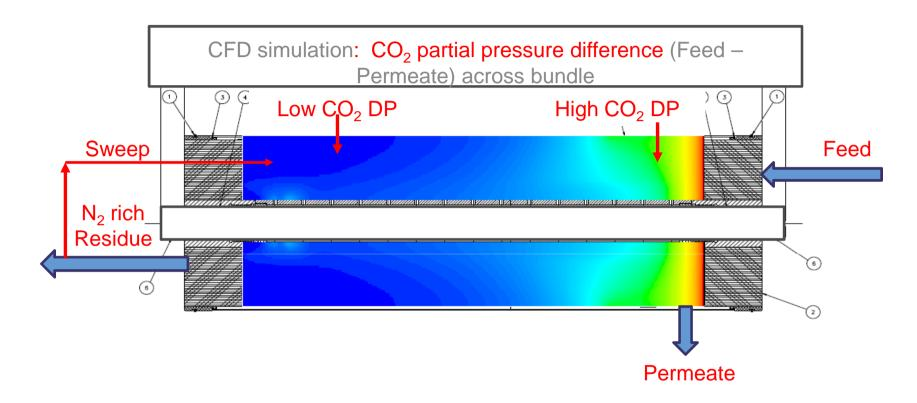
Addition of Sweep increases driving force across membrane for efficient flue gas separation
