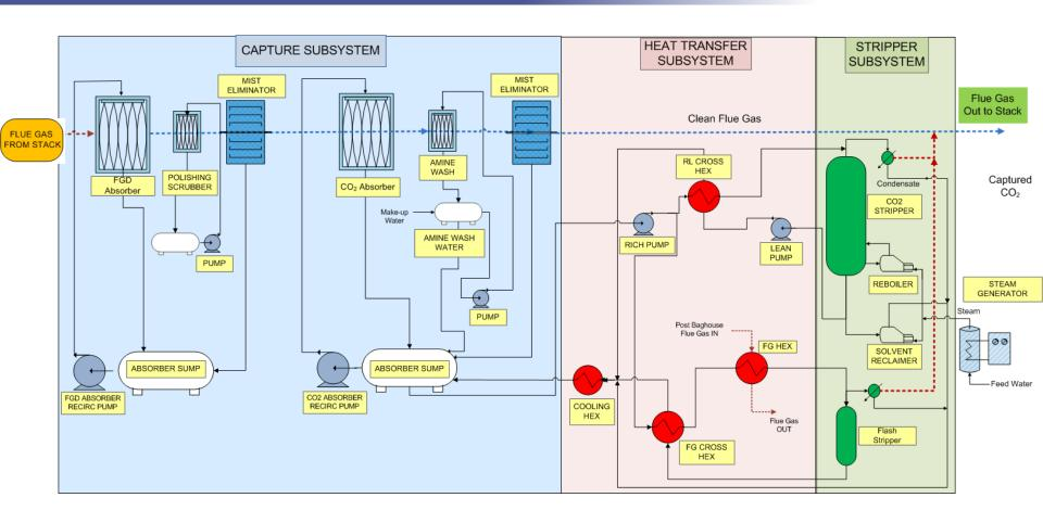
NSG flat jets are incorporated into the FGD, Polishing FGD, CO<sub>2</sub> Absorbers, Amine Wash, and Stripper
