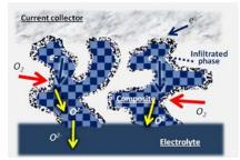
Cathode infiltration technology is being developed to enhance the SOFC operating performance. Initial results have demonstrated > 40% performance improvement and acceptable material stability.
