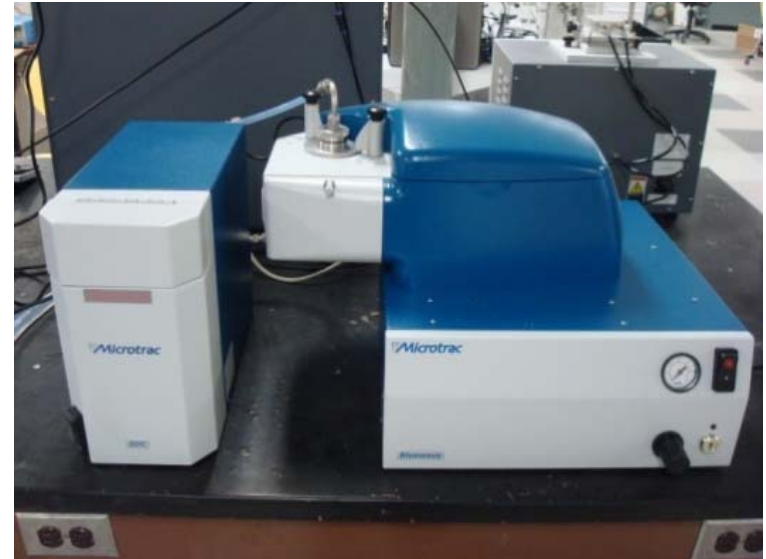
Multi-laser particle size analyzer (Microtrac Bluewave)
