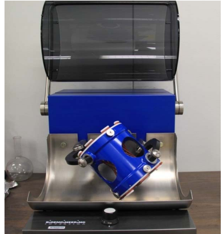
Three-dimensional inversion kinematics tumbler mixer (Inversina 2L)
