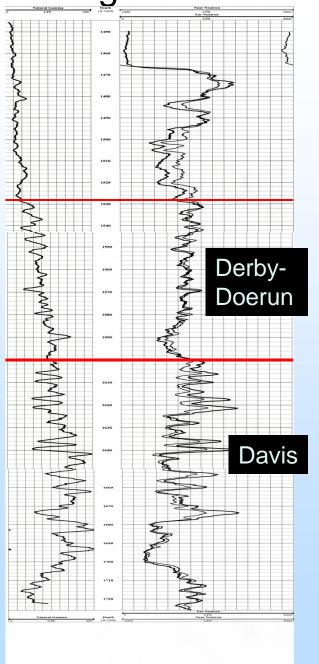
St. Francois confining unit is about 50% shale; carbonates are mostly discrete clasts within shale.
