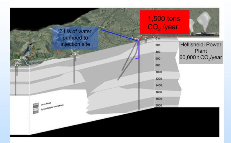
distance between injection and first monitoring well is 150 m
