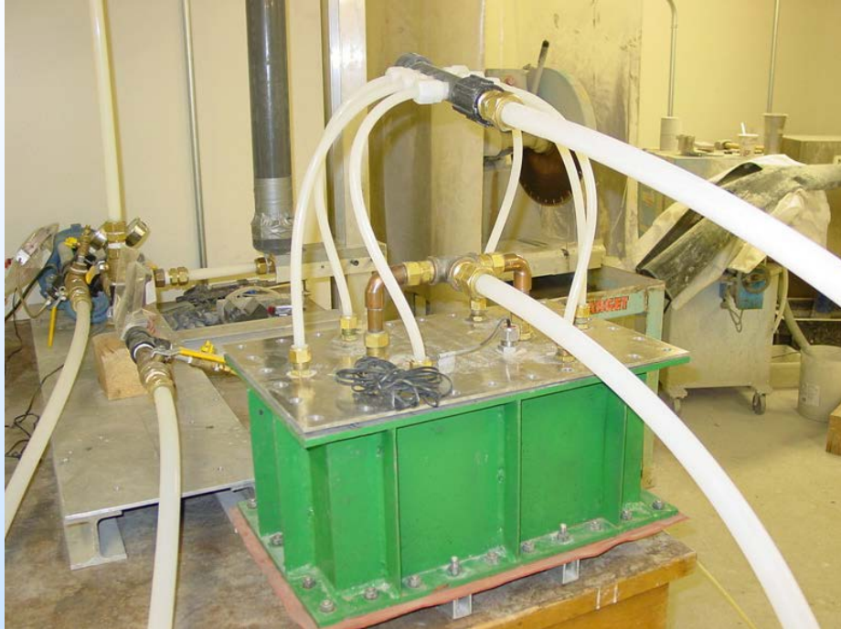
Single block CO 2 Clave for both static and dynamic carbonation
