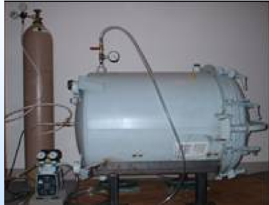
CO 2 Clave for static carbonation of multiple 8"-blocks or 1'x2' panels
