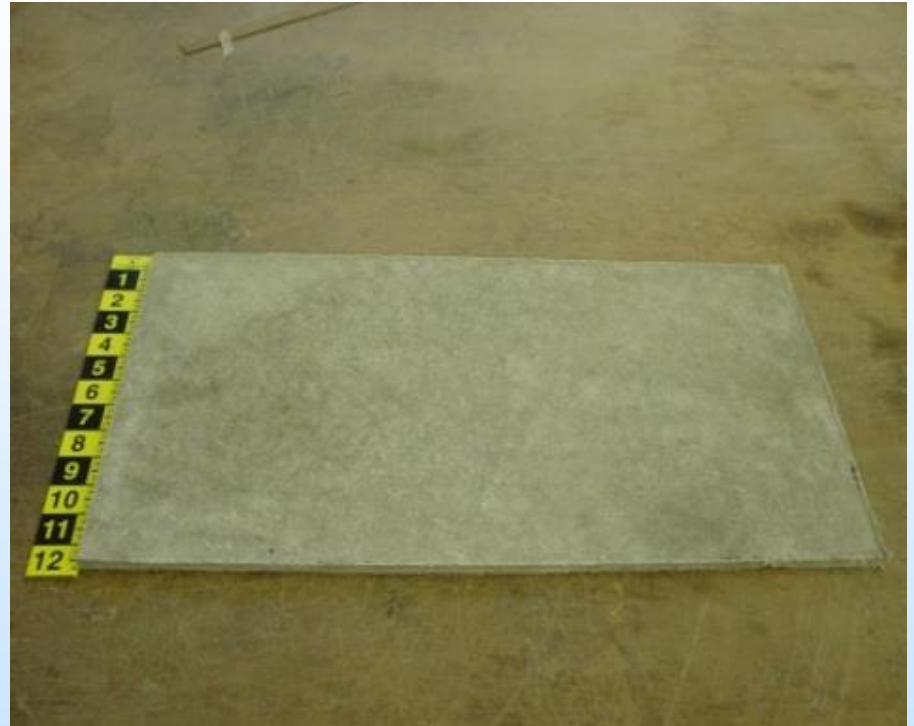
1'x2' fiber cement panel (0.5" thick) Target: 0.65 lb CO 2 per 1'x2' panel
