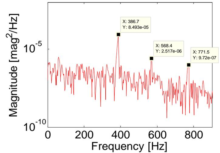
PSD of Pressure at Jet Injection
