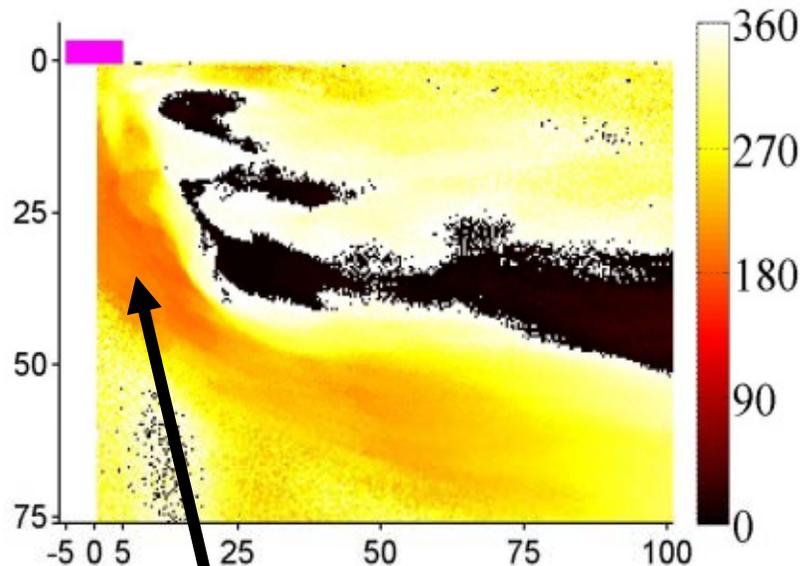
Windward side of jet in phase with downstream running compression wave
