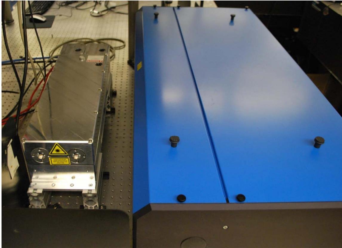
Edgewave Diode-Pumped Solid State Nd:YAG Laser: 5 kHz Rep Rate, Dual-Head, 6 mJ/Pulse at 532 nm, 7 nsec Pulses
