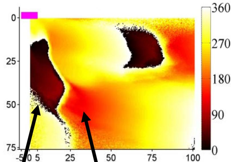
Periodic jet tip in phase with mean flow maximum ( $u'$  with mean flow)
