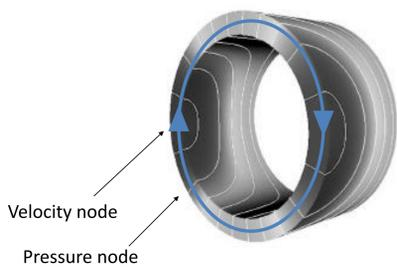
Figure 2a. Acoustic model for an annular geometry[2].
