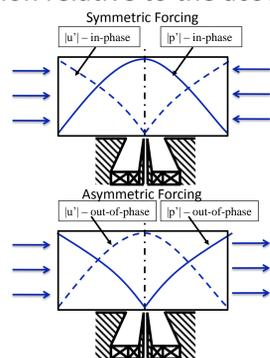
Figure 2b. Acoustic oscillations for pressure anti-node (top) and pressure node (bottom).
