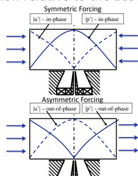
Figure 2b. Acoustic oscillations for pressure anti-node (top) and pressure node (bottom).
