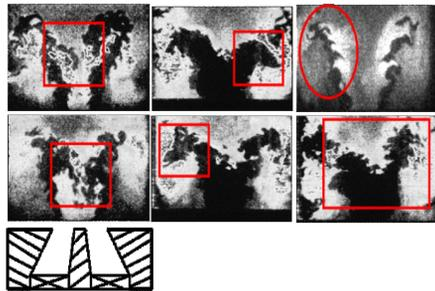
Figure 1b. Planar-laser induced fluorescence (PLIF) depicting flame wrinkling from acoustics excitation[1].
