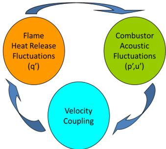
Figure 1a. Coupling process during combustion instabilities.
