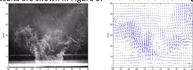
Figure 5. Raw particle image (left) and vector field (right) from HSPIV laser diagnostic tool.
