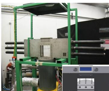
Figure 3. Facility for transverse combustion instabilities.
