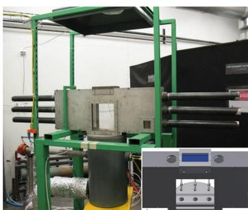
Figure 3. Facility for transverse combustion instabilities.
