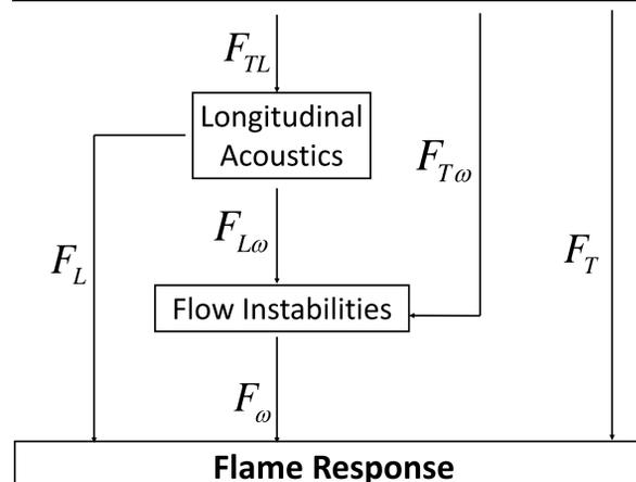
Figure 6. Possible flame response pathways during transverse forcing for swirl-stabilized flames.
