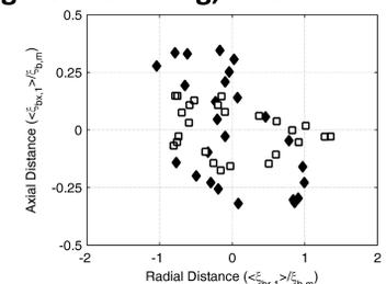
Figure 8. Forced flame motion normalized by particle motion for symmetric forcing (solid) and asymmetric forcing (open).
