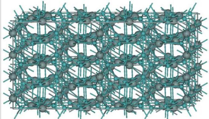
**Orthorhombic 256-atom supercell model of  $\text{Mo}_5\text{Si}_3$  used for tensile experiment for failure envelope.**
