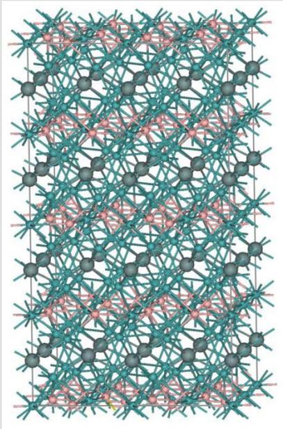
**Orthorhombic 256-atom supercell model of  $\text{Mo}_5\text{SiB}_2$  used for tensile experiment for failure envelope.**
