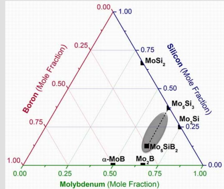
Phase diagram within Mo-Si-B system. Four composite models between the two crystalline phases  $\text{Mo}_5\text{Si}_3$  and  $\text{Mo}_5\text{SiB}_2$  are studied based on the crystal framework of  $\text{Mo}_5\text{SiB}_2$ .
