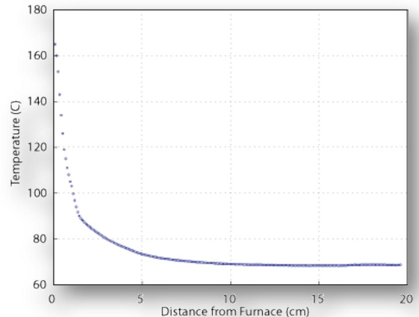
Temperature declines rapidly down the length of the cylinder from the furnace
