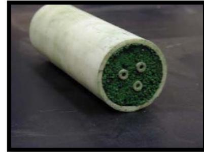
Thermocouple protection system for gasifier application [2].
