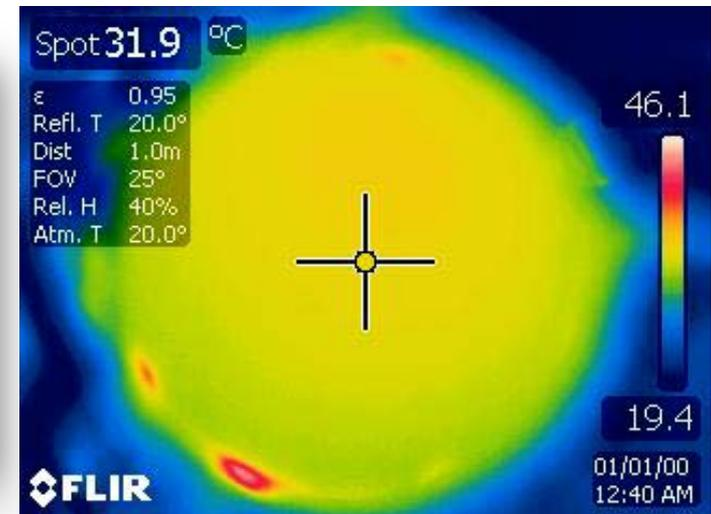
Thermal imaging suggests that heating inside laboratory oven is axially symmetric.
