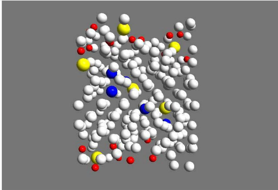
**O/Cr-Y-Mo system at 1200 K with O atoms diffused. 238 Cr atoms (White), 6 Y atoms (Yellow), Mo atoms (Blue) and 21 O atoms (Red) are shown in the figure.**
