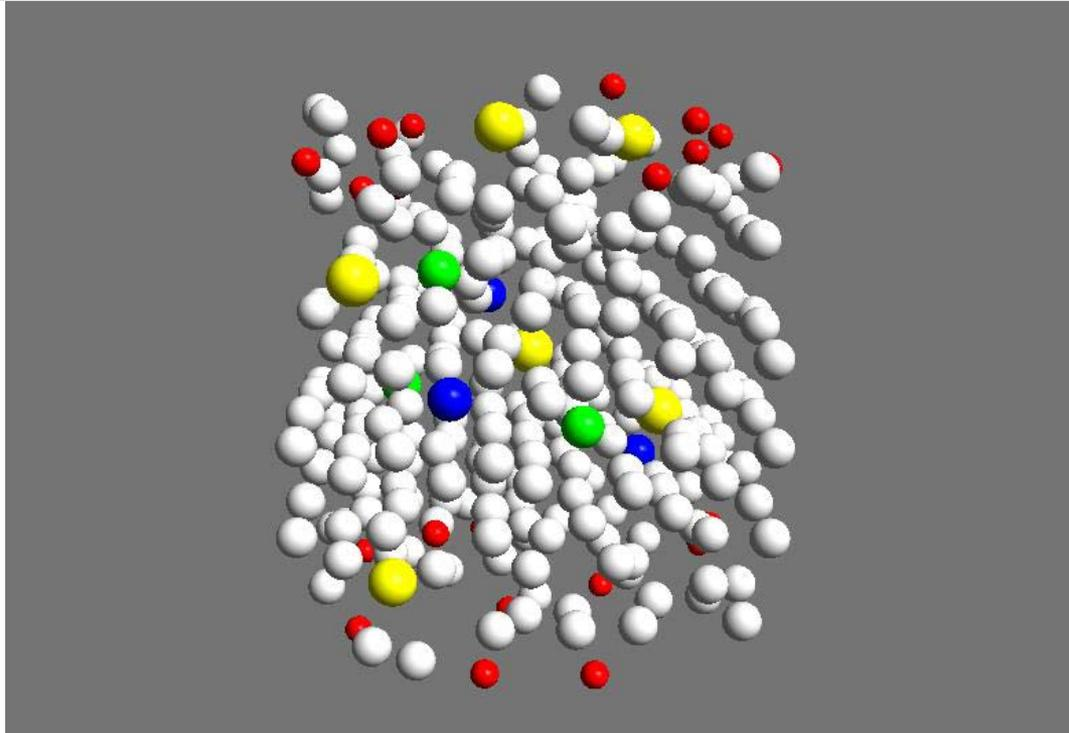
**O/Cr-Y-Mo-W system at 1200 K with O atoms diffused. 238 Cr atoms (White), 6 Y atoms (Yellow), 3 Mo atoms (Blue), 3 W atoms (green) and 21 O atoms (Red) are shown in the figure.**
