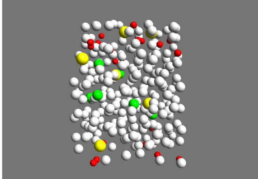
**O/Cr-Y-W system at 1200 K with O atoms diffused. 238 Cr atoms (White), 6 Y atoms (Yellow), 6 W atoms (Green) and 21 O atoms (Red) are shown in the figure.**
