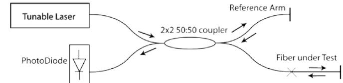
**Fig. 3:** Schematic sketch illustration of the OFDR operation principle [20].
