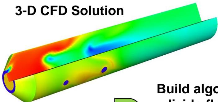
Build algorithm to divide flow field into reactor zones
