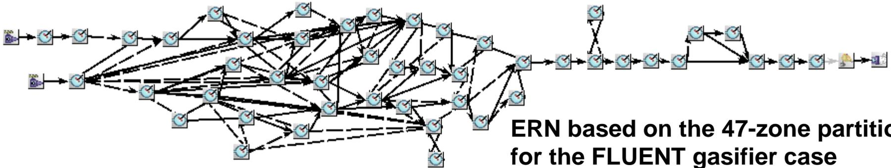
ERN based on the 47-zone partition for the FLUENT gasifier case
