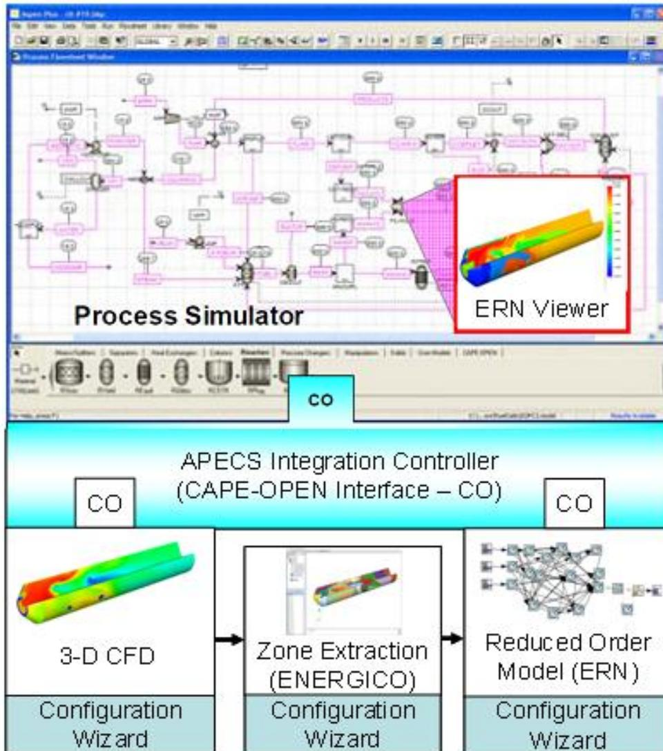
Co-simulation project involving flowsheet simulation, CFD simulation, and Reduced-order Models (ROMs)
