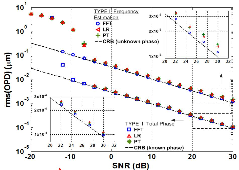
↑ Improved signal processing reaches the theoretical limit of resolution<sup>[1]</sup>
