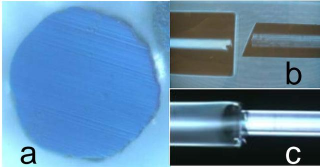
↑ a. Sapphire fiber angle-polished end face. b. sapphire-silica splicing. c. splicing point with angle-polished sapphire fiber.
