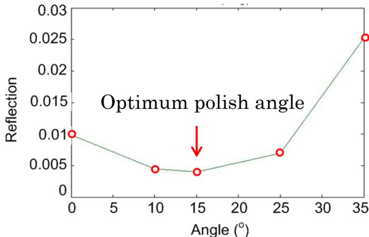
← Result showing the determination of the optimum polishing angle to yield minimum back reflection.
