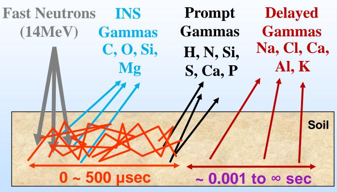
**Neutrons Thermalize via Delayed Activation Elastic Scatterings and Following Neutron Thermal Neutron Captures**
