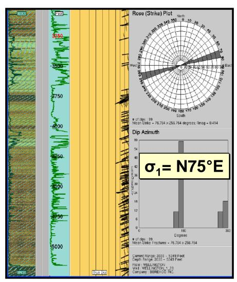
There are 99 drilling induced fractures in this pass, oriented  $76^{\circ}/256^{\circ}$ , indicating the maximum stress direction.
