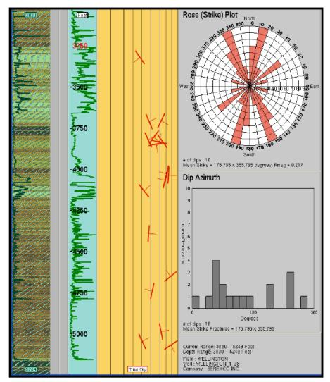
There are 18 natural mineralized "closed" fractures in this pass with two orientations, the first is NNE x SSW and the other is NNW x SSE.
