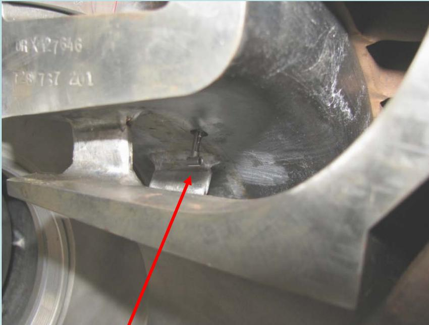
Combination Kiel Head Pressure/Temperature Probe at Suction and Discharge Bridge-over
