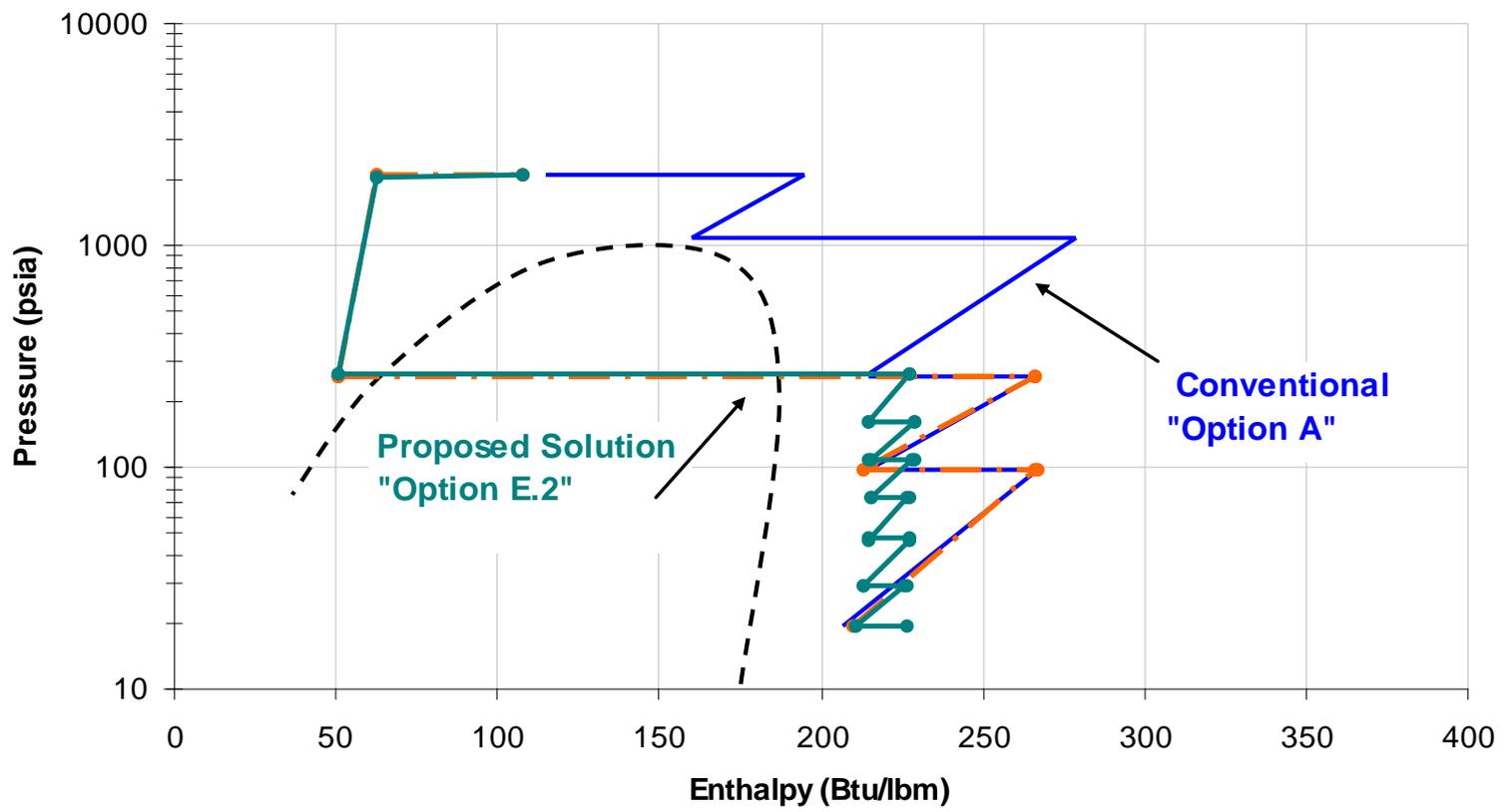
Optimal solution combines inter-stage cooling and a liquefaction approach.
