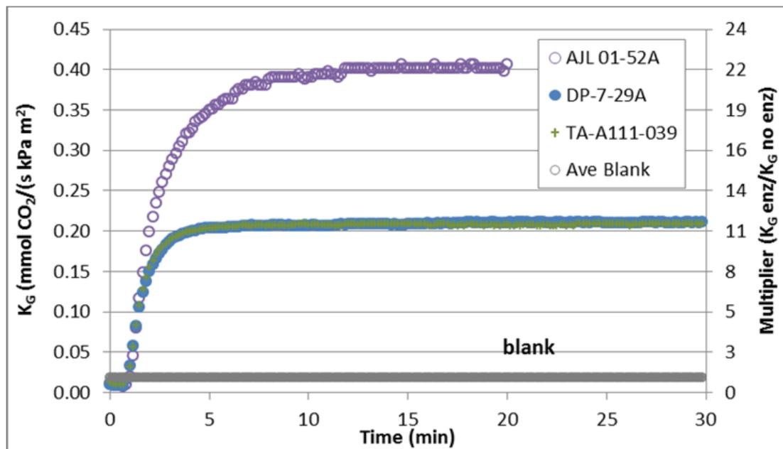
$K_G$  per packing area, lab-scale test reactor interfacial area ~ 30%
