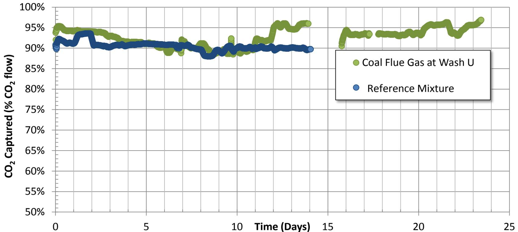
~ 90-95% CO<sub>2</sub> capture sustained for over 23 days on flue gas (~14% feed)
